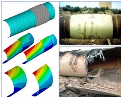
3 – Crack arrestor for fracture arrest.
